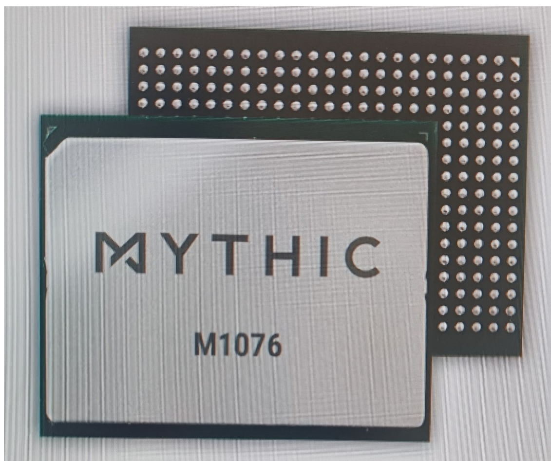
Figure 5: Analog mother processor that delivers analog computing for artificial intelligence that is comparable to a digital device with precision and power, MYTHIC, Austin, Texas, 2012, ( https://mythic.ai )
