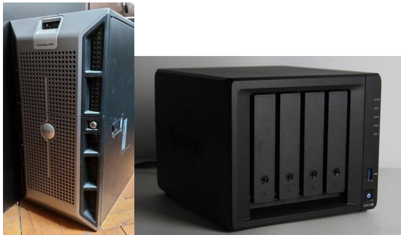
Photo 8 and 9 - Server Dell PowerEdge 2900 and Network-Attached Storage Synology DS920+ in use in the Archives of Bosnia and Herzegovina
